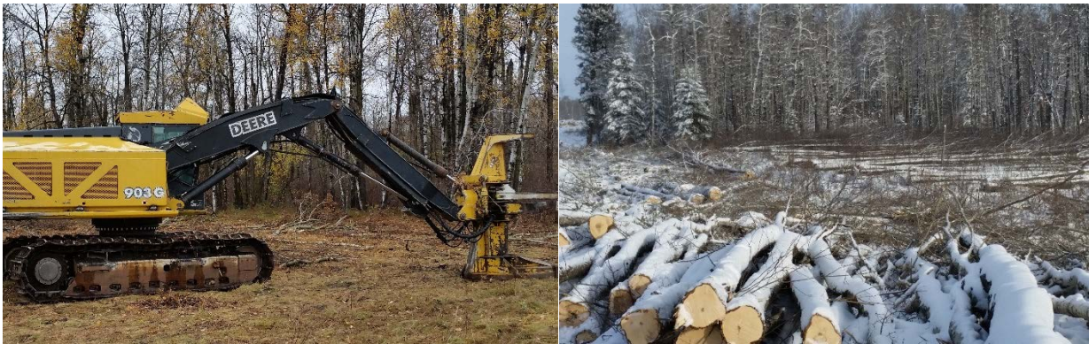
Figure 6.15 Feller-buncher machine (left) and bunches of tree length ready for skidding.
