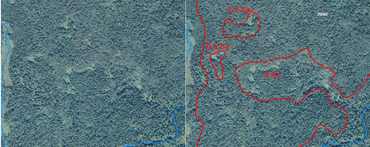
Figure 6.8 Southern tip of the Silver creek block appears all operable (left) but has non-operable areas that are manually removed (red polygons on right).
