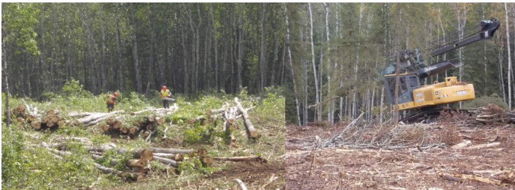
Figure 6.16 Topping and limbing with power saws (left) and a stroke delimiter (right).
