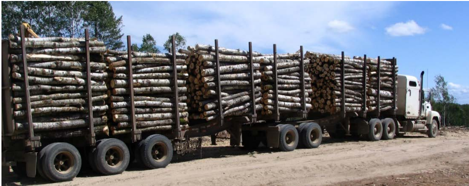
Figure 6.20 Super B haul trailer with a load of 2.5 m aspen bolts.
