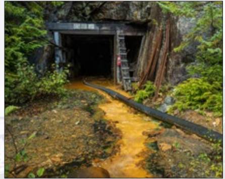
Photo: Acid mine drainage pours from Tulsequah Chief mine opening (Chris Miller - csmphotos.com).
